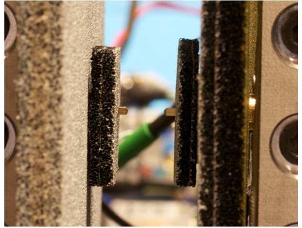
Fig. 3: Photo of the antennas used in the system. The antennas are open-ended waveguides and the walls of the waveguides have been cut in a 45^\circ to minimize the effects of standing waves between the fronts of the antennas. For the same reason, absorbers (seen as gray and black material on the photo) are mounted around and behind the antennas.
