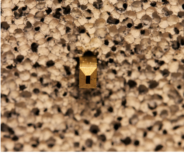
Fig. 4: Close-up of one of the antennas in the system. The opening of the waveguide measures 0.355 mm by 0.710 mm and the walls of the waveguide has a thickness of 0.500 mm.
