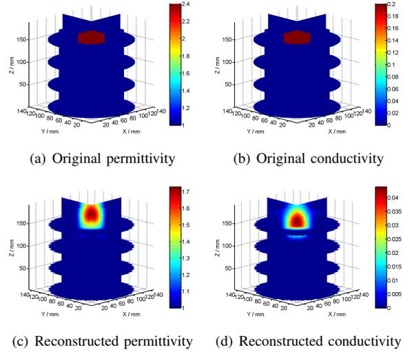
Fig. 2. (a) Original relative permittivity of the test object, (b) and original conductivity of the test object. (c) A reconstruction of the relative permittivity (d) and a reconstruction of the conductivity.
