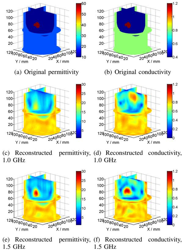
Fig. 3. (a) Original relative permittivity and (b) conductivity of the breast model. In (c) a reconstruction of the relative permittivity and in (d) the conductivity using a pulse with center frequency 1.0 GHz and FWHM bandwidth 1.0 GHz. In (e) and (f) the results from continued reconstruction using center frequency 1.5 GHz and FWHM bandwidth 1.0 GHz with the images from (c) and (d) as the starting point.
