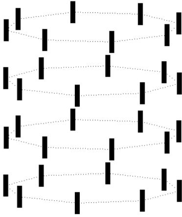
Fig. 1. The principal design of the antenna array for a clinical microwave tomography system. The antenna array consist of 32 antennas on total, configured in four circles with eight antennas in each circle.
