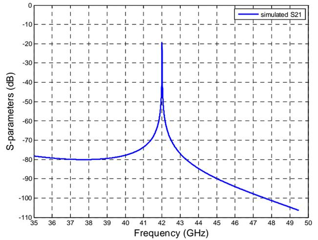
Fig.4 Ridge gap waveguide resonator frequency response
