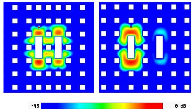
Fig. 6 Changing in coupling of two ridge gap resonators by changing 's'
