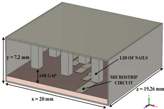
Fig.12 Microstrip Coupled line 3<sup>rd</sup> order filter with pin lid package
