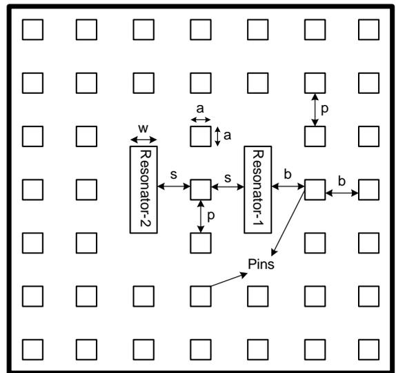
Fig. 5 Coupling of two ridge gap resonators
