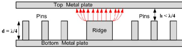
Fig.1 Ridge gap waveguide geometry.
