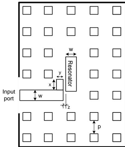
Fig. 8 Excitation of the input and output ridge gap resonator
