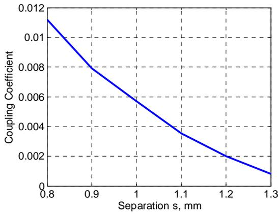
Fig. 7 Coupling coefficient 'k' vs 's'
