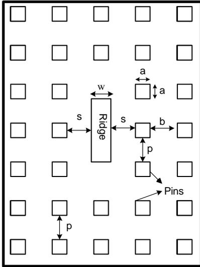
Fig.2 Ridge gap waveguide resonator,  $a = 0.8\text{mm}$ ,  $w = 1\text{mm}$ ,  $p = 1.25\text{mm}$ ,  $s = 1\text{mm}$ ,  $b = 1.35\text{mm}$ , top metal plate not shown.
