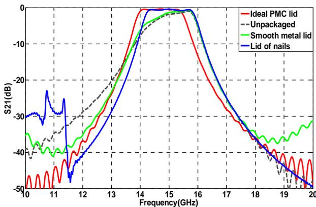
Fig.12 Microstrip filter response for different packaging cases
