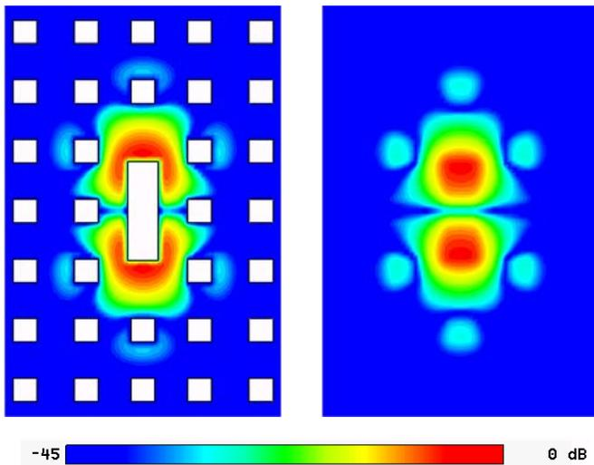
Fig. 3 Vertical E field distribution within a ridge gap resonator
