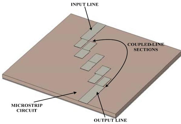
Fig.11 Microstrip Coupled line 3<sup>rd</sup> order filter
