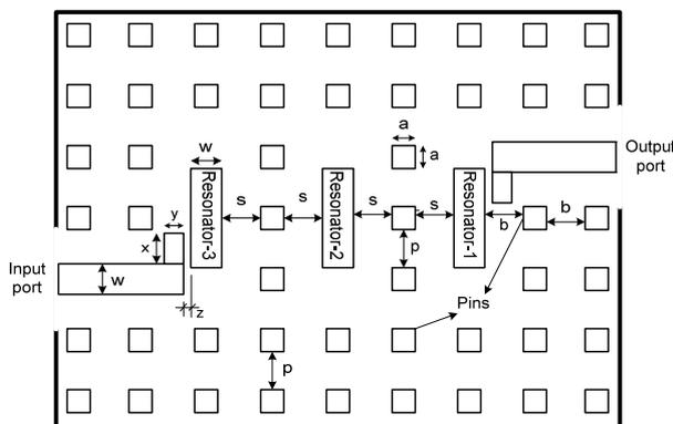
Fig. 9 Complete 3<sup>rd</sup> order filter geometry
