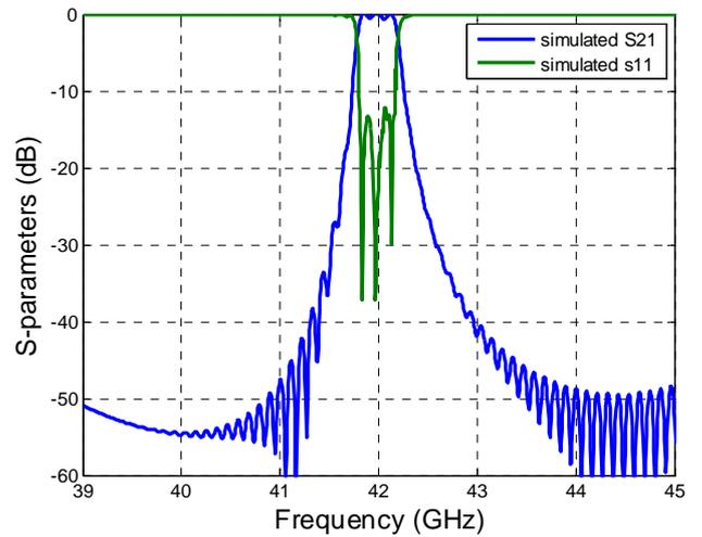
Fig.10 Simulated S parameters for the 3<sup>rd</sup> order filter
