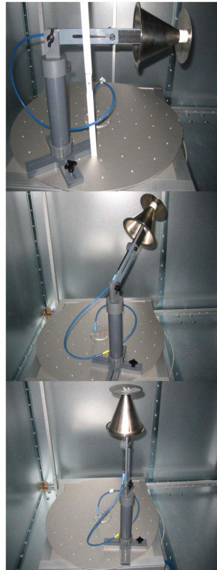
Fig. 3 The three different orientations (horizontal, 45 degree and vertical) of the receiver antenna used for the system validation procedure. These orientations are repeated for three different heights over the turntable, 30, 38 and 46 cm, giving a total of nine different receiving antenna positions.
