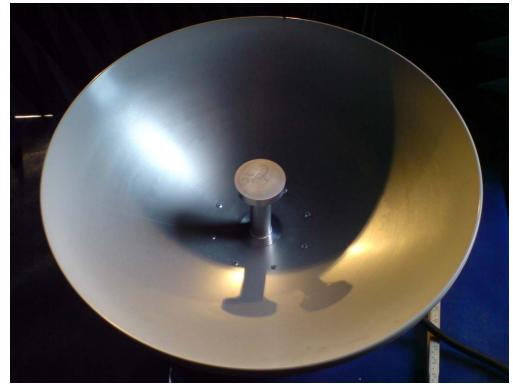
Fig. 7. The new hat feed mounted in a reflector with a diameter of 654 mm and a subtended angle of 105°.
