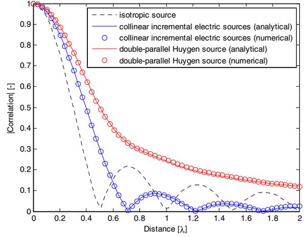
Fig. 2 Comparison of the normalized correlations of incremental electric source pair in collinear arrangement and Huygen's source pair in double-parallel arrangement, calculated numerically and analytically, together with that of isotropic source.
