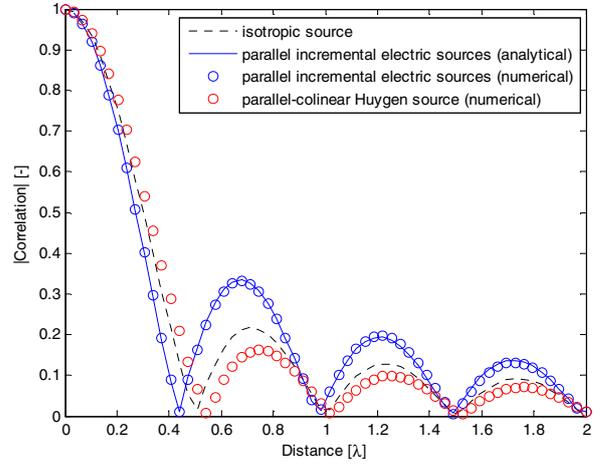
Fig. 3 Spatial correlation for parallel incremental electric source and parallel-collinear Huygen's sources, together with that of isotropic source.
