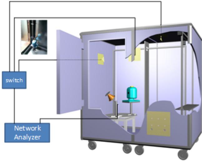
Fig. 4 Drawing of Bluetest RC with two mechanical plate stirrers, one platform and three wall antennas.
