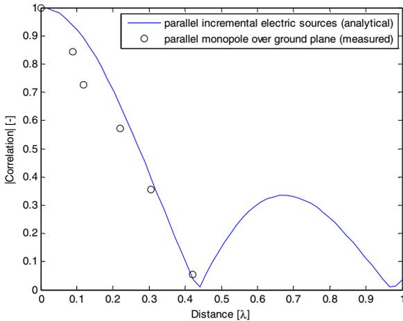
Fig. 6 Measured spatial correlation of parallel monopole in reverberation chamber against that of theoretical parallel incremental electric source.
