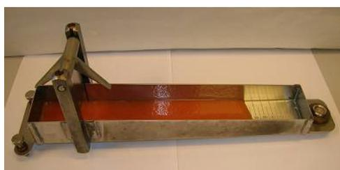
**Figure 5.** *The Bostwick consistometer used in studies 1 and 2. The gate to the left has been opened and tomato pulp is running down the graded slope. The Bostwick consistency index is determined as the distance the pulp has run down the slope after a set time.*
