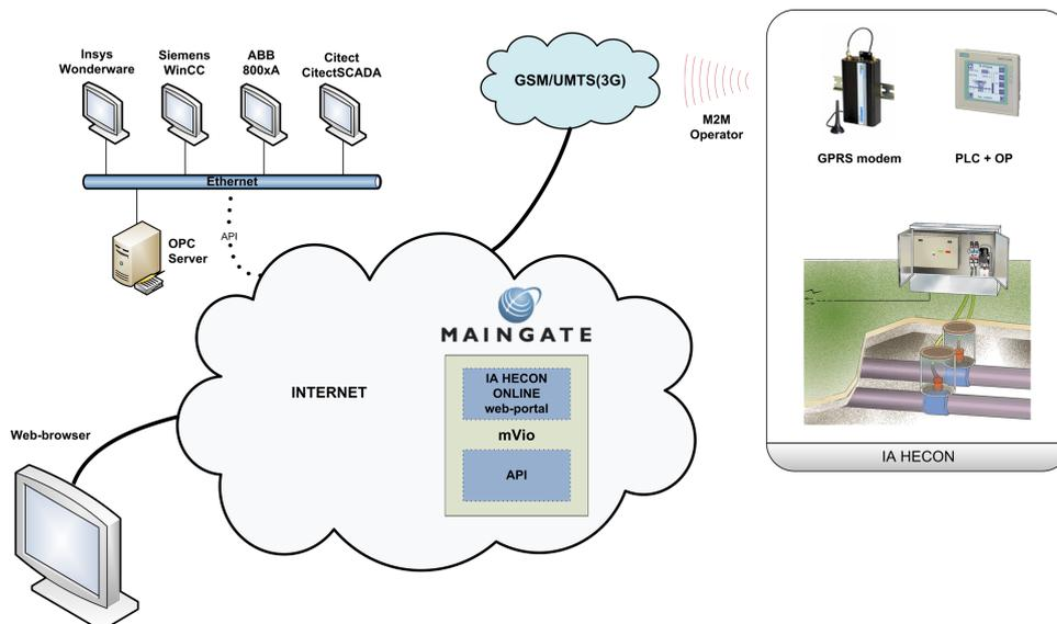
Figure 4.3: mVio Internet SCADA, architecture
