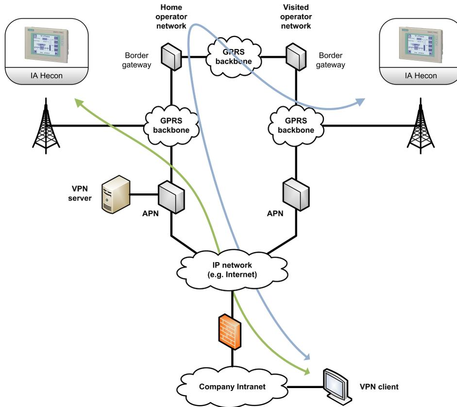
Figure 3.7: GSM and GPRS architecture
