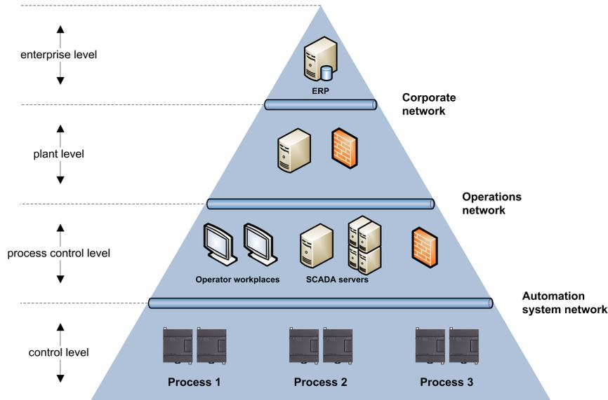
Figure 3.3: Industrial control system architecture
