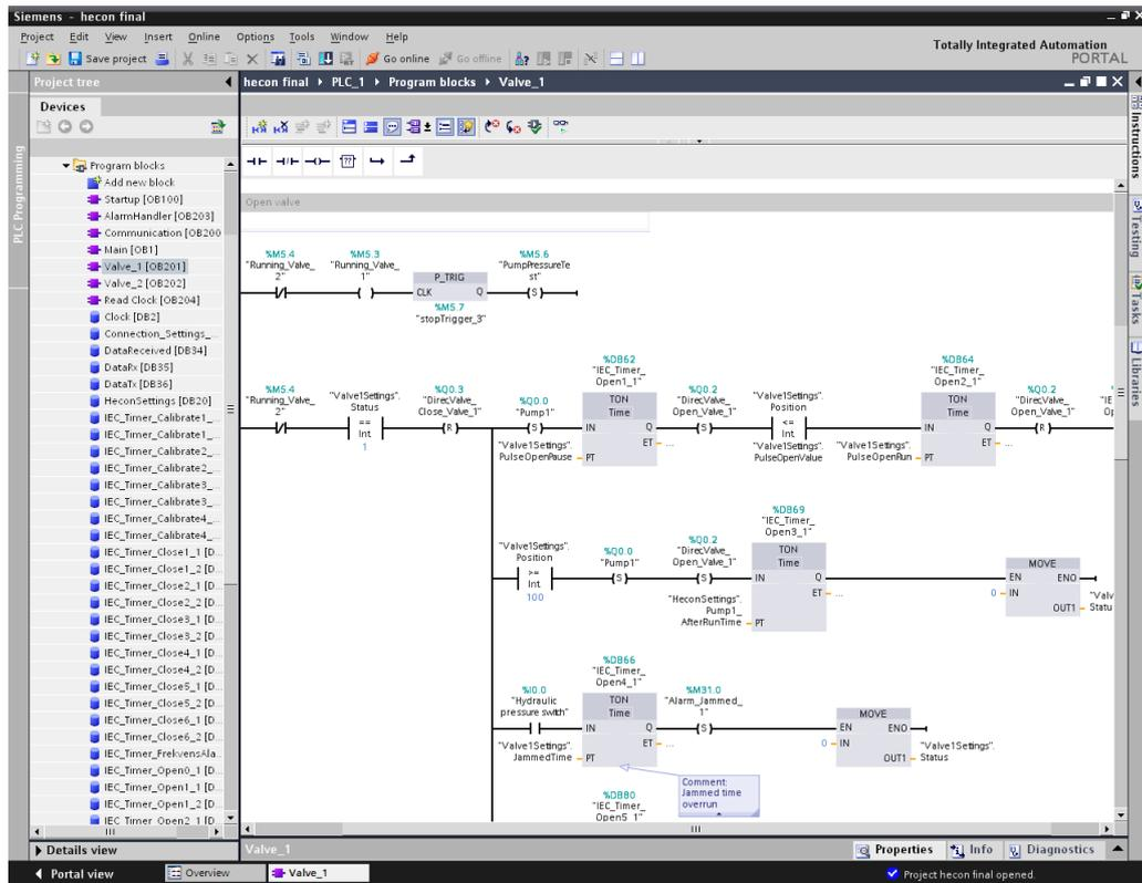
Figure 5.4: PLC ladder code example
