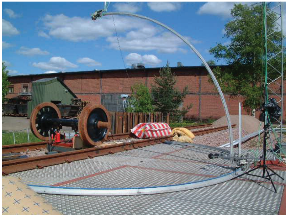
Fig. 2.1. The Railway Noise Test Rig at Lucchini Sweden in Surahammar
