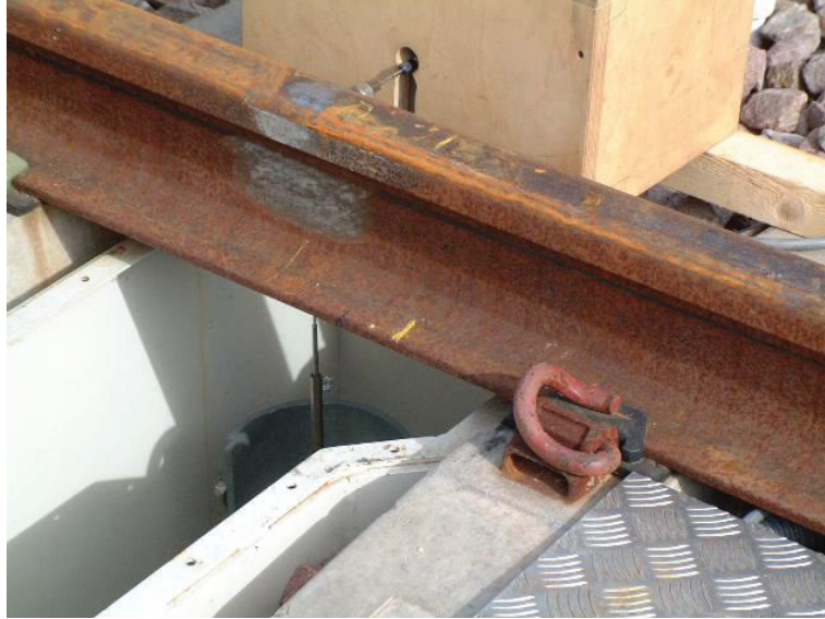
Fig. 2.2. The vertical and lateral force actuators
