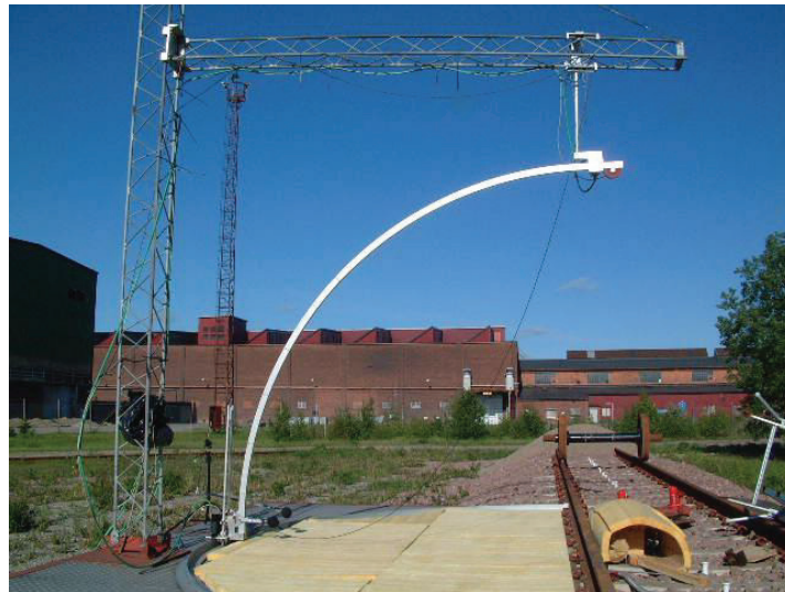
Fig. 2.6. Measuring vertical directivity of rail radiation at the RNTR in Surahammar
