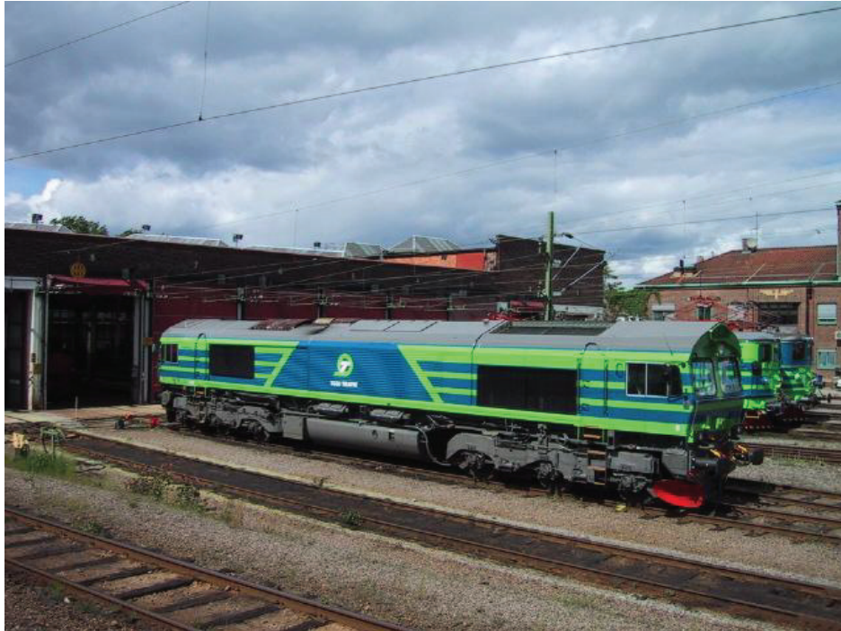
Fig. 2.14. The measured diesel-electric locomotive of GB T66 type. In the picture the long-side 2 is shown, which was facing the sea when its sound power was measured.
