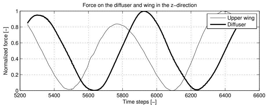
Figure 57: A comparison of the normalised force, in the z -direction, acting on the upper wing and on the diffuser over a time period of two full wheel revolutions
