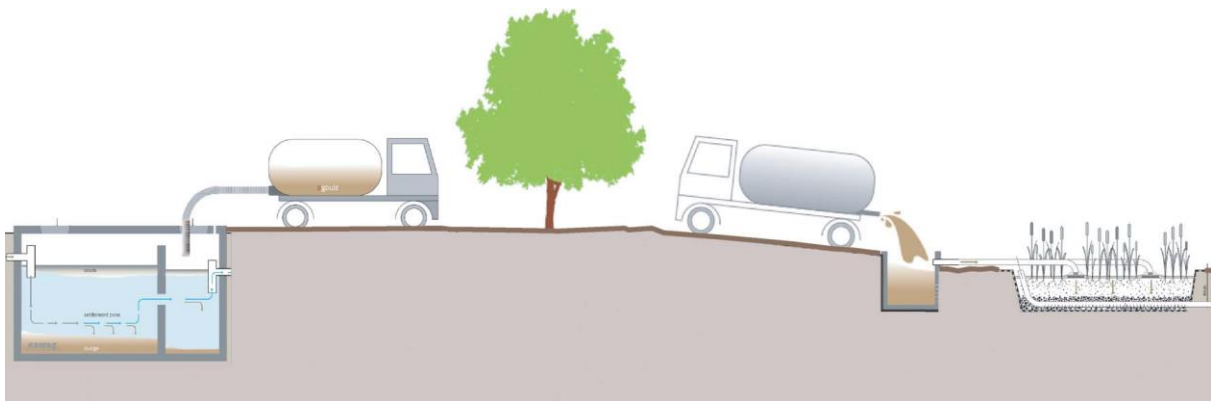
Figure 3: HCES consider the entire sanitation system and a variety of technical options that are available from the toilet to the final treatment. Example of a sanitation system configuration involving storage (septic tank), transport (motorized emptying) & treatment (constructed wetland).
