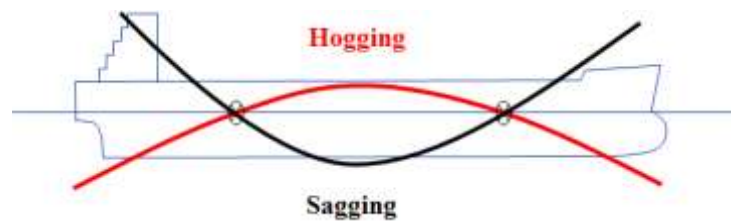
Figure 1.1, Vertical 2-node vibration of ship structure
