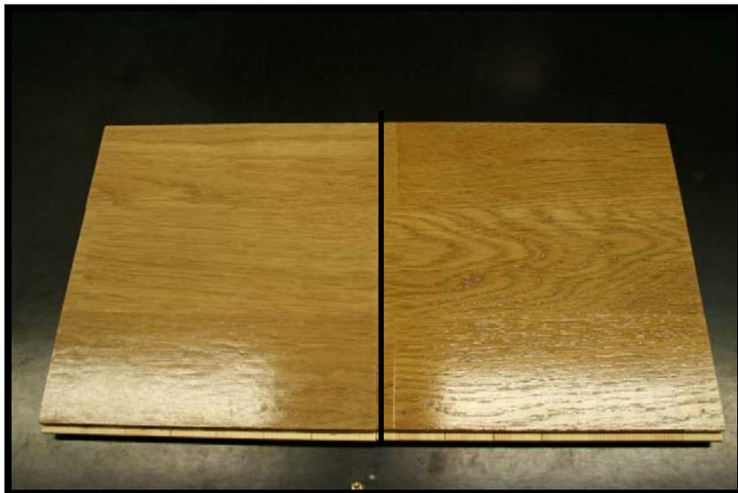
**Figure 14: 1-pack water-based lacquer formulated on acrylic resin without (left) and with (right) 20% SiO<sub>2</sub> addition of epoxy-silane modified colloidal silica.**
