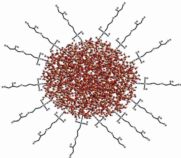
Epoxy silane-modified colloidal silica particle. The particle size of the silica core is 7 nm.
