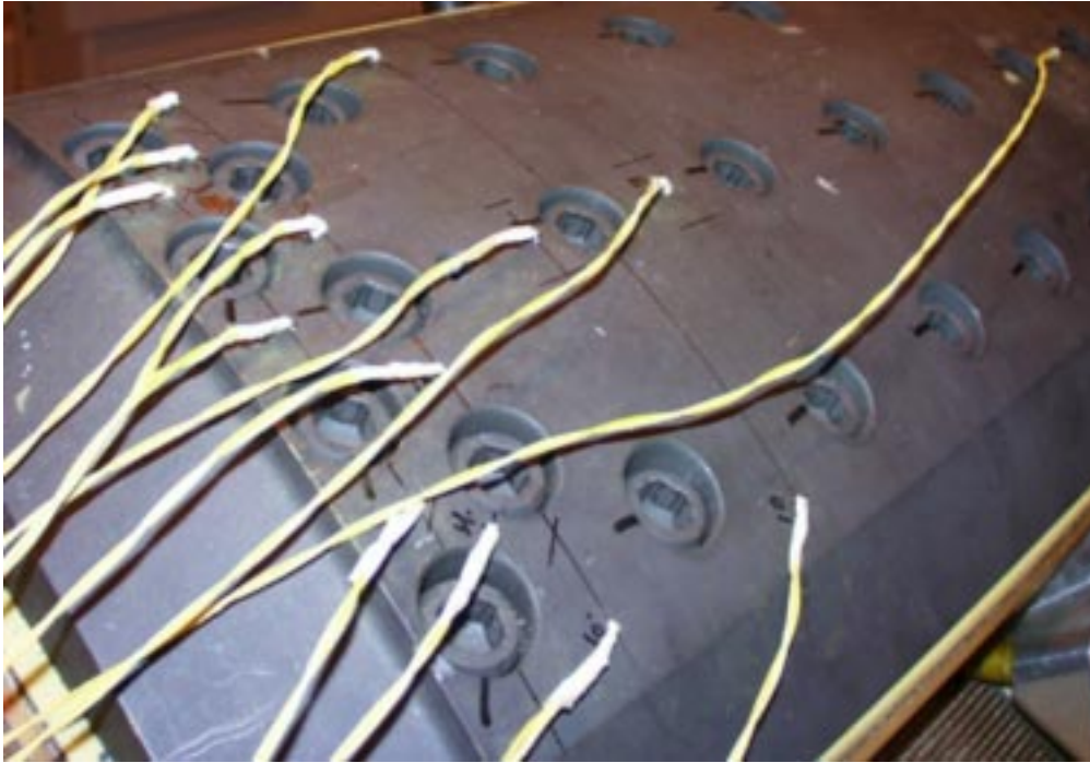
Figure 5.43 Some thermocouples on the rotor surface.
