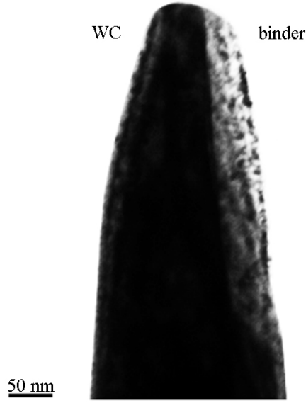
Figure 23: TEM micrograph of an analysed APT specimen with a WC/binder phase boundary. Note the larger tip radius on the binder phase side.
