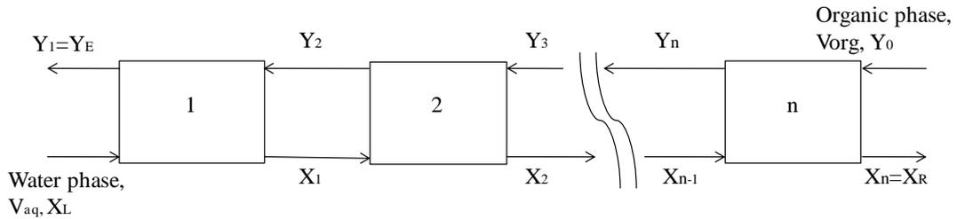
Figure 3.5. Solvent extraction process using counter-current flows in  $n$  steps.  $Y_0$  refers to the initial amount of Cu in the organic phase, while  $Y_E$  refers to the amount in the loaded organic phase.  $X_L$  refers to the initial amount of Cu in the water phase and  $X_R$  refers to the amount of Cu after  $n$  extraction steps.
