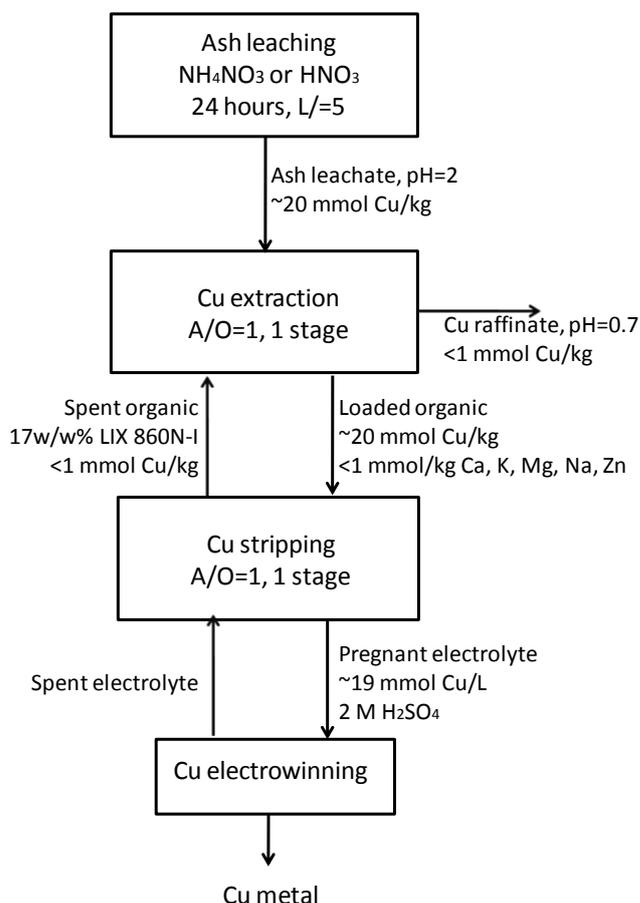
Figure 5.17. Flow sheet of the recovery method developed for Cu from ash.
