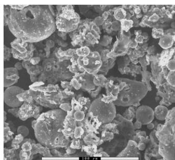
Figure 5.4. SEM image, 500x magnification, of the size fraction with particles  $>180\mu\text{m}$  in ash D. The bar corresponds to  $100\mu\text{m}$  (Paper II).
