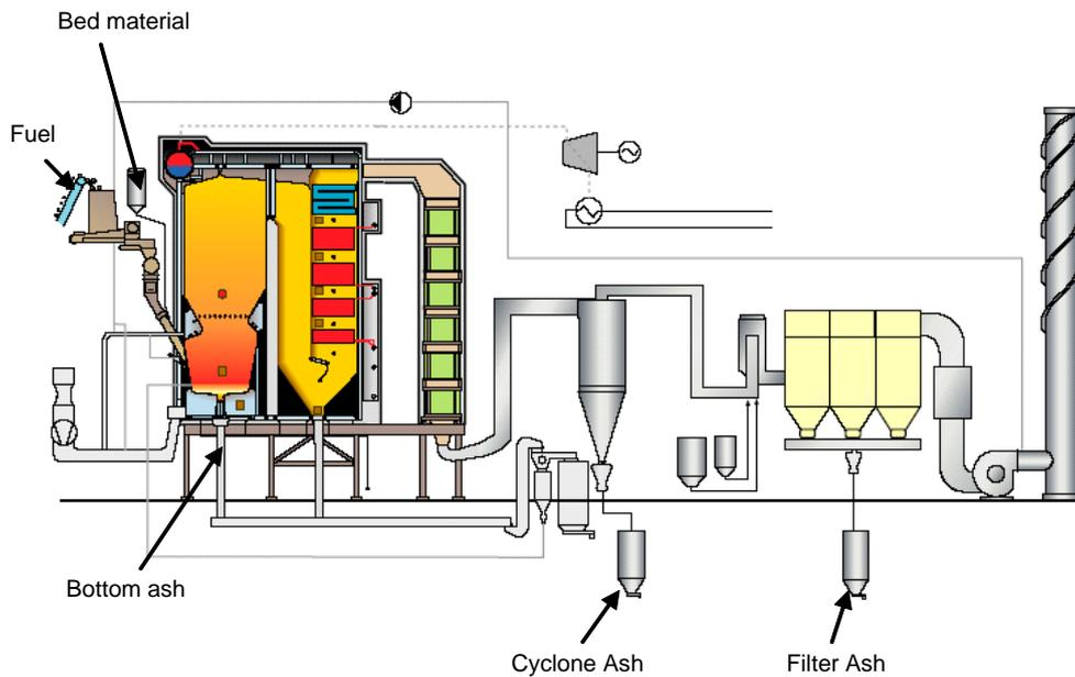
Figure 3.2. Schematic picture of a bubbling fluidised bed combustor. Printed with the permission of [20].
