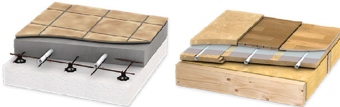
**Figure 2** Illustration of a floor heating construction. On the left-hand side a concrete embedded system and on the right-hand side a light weight system with heat conduction plates fitted in a wooden joist. (By courtesy of Uponor)
