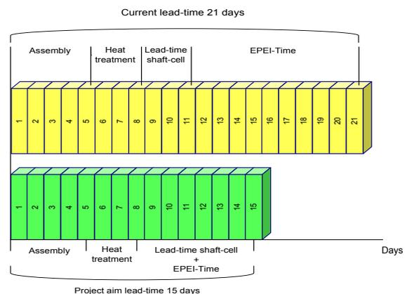
**Fig 1: Current state at the case study company versus desired situation to be able to keep the promised lead-time to customers.**
