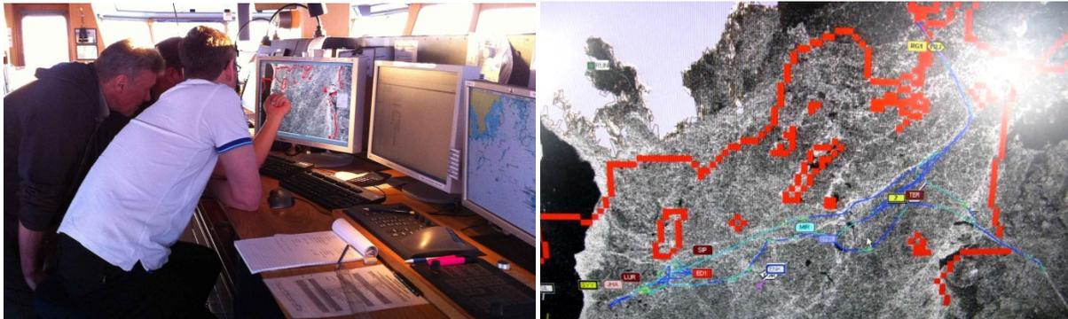
Fig.5. Left: the bridge crew is gathered in front of the IBNet screen, studying a fresh satellite picture. Overlaid on the satellite picture are the 10 meter safety contour (red), the prevailing wind, and the different ships in the area, ice breakers, and ordinary vessels color coded for their port of destination and with tracks color coded for speed.
