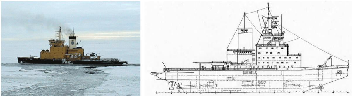
*Fig. 1. The Swedish Maritime Administration's icebreaker Frej. Three Swedish ships of this class were built 1974-77 by Wärtsilä ship yard in Finland (and also three Finnish ships of the same class, the blueprint is of the Finnish sister ship Sisu).*
