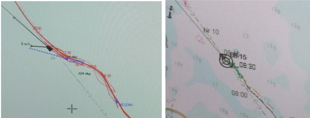
Fig.7. Left, a screen shot from the Adveto ECDIS, the ice breaker is escorting a convoy of two ships at 8.45 in the morning. He is using the historic track of himself from about 23.00 the previous night, showing that the ice sheet has been stable and not drifting. To the right is a screen shot from the regular Furuno ECDIS a little earlier. The historic track cannot be called up here.
