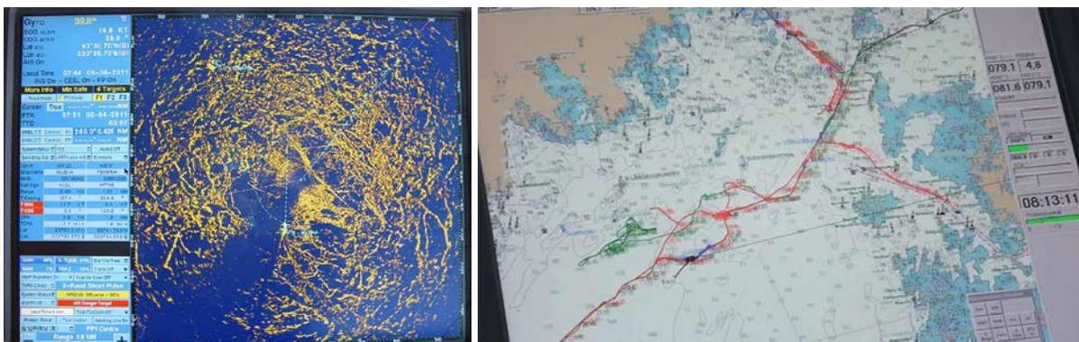
Fig.6. Left, the Consilium Selesmar ice radar and right, the Adveto ECDIS. Past track of several recent vessel movements gives a view of open ice channels in the area.
