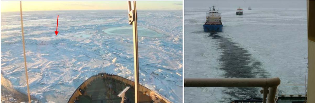
Fig. 2. Left, *Frej* is opening a new channel through the 30-55 cm thick ice. By the red arrow she is brought to a complete stop by this seemingly insignificant ice ridge that shows very little of its true size above the ice sheet. Right, convoy service. Often the ships in the convoy get stuck and the ice breaker has to go back and break them free. During this maneuver, the other ships get stuck. It is a tedious work.
