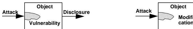
Figure 4: Two attacks against an object resulting in a) disclosure b) modification of information
