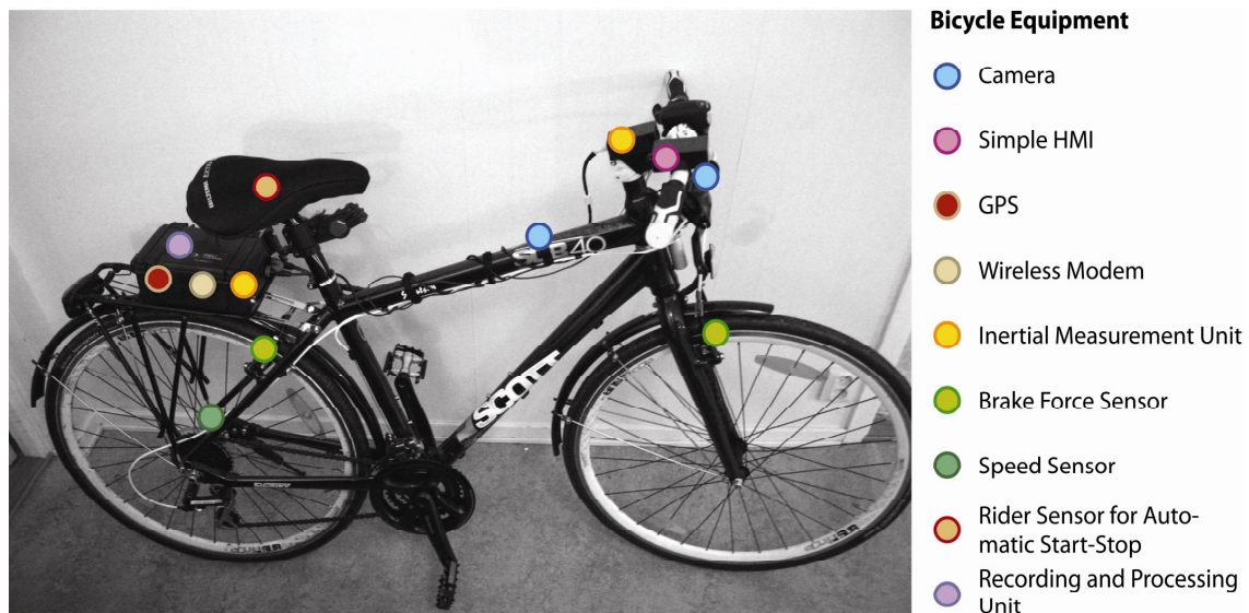
Figure 3. Instrumented bicycle for analysis of naturalistic cycling data.
