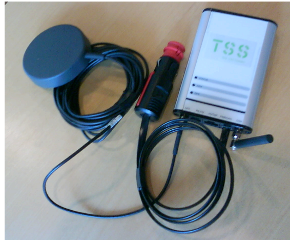
Figure 7: The GPS equipment is contained in a box with antenna for gprs communication and supported with a GPS antenna (left) and plug for 12 V outlet.
