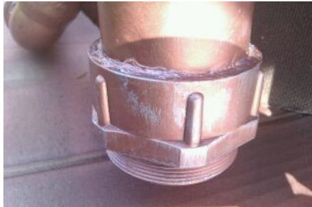
Figure 3: Shows paint detail and the fake welding.
