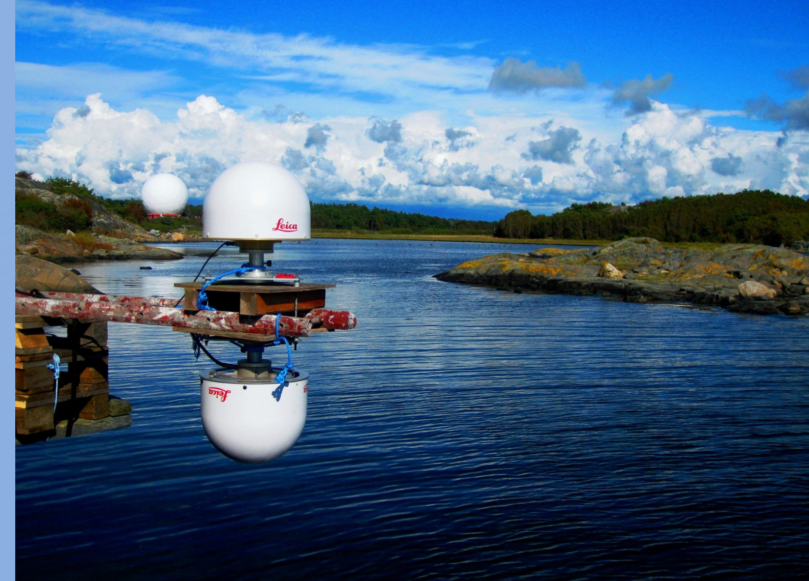
Figure 1 – The GNSS-based tide gauge at OSO.
