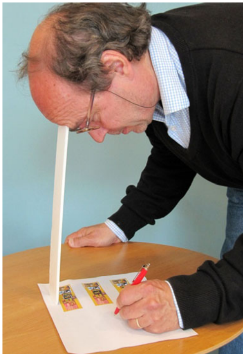
Fig. 6 One of the authors demonstrates how the measurements were conducted (here experiment 2): A 32 cm high support made sure the distance to the stimuli was the same for all participants. The subject fixated the tip of a ballpoint pen starting at the target sign and then moved the pen left away from the target until the target could no longer be seen in the corner of the eye. That point was then marked on the paper and the distance entered as the conspicuity index
