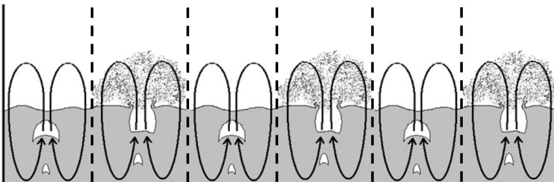
Figure 1: Horizontally aligned solid transport vortices, induced by the formation of stable bubble paths. Particles are ejected at the surface when a bubble erupts. The flow domain can be divided into discrete regions which are indicated by the dashed lines. Based on findings by Pallarès and Johnsson (2006).
