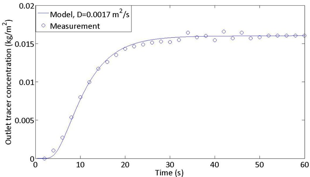
Figure 3: Results from a run at  $U_0 = 0.37 \text{ m/s}$ . The dispersion coefficient was determined to  $0.0017 \text{ m}^2/\text{s}$ .
