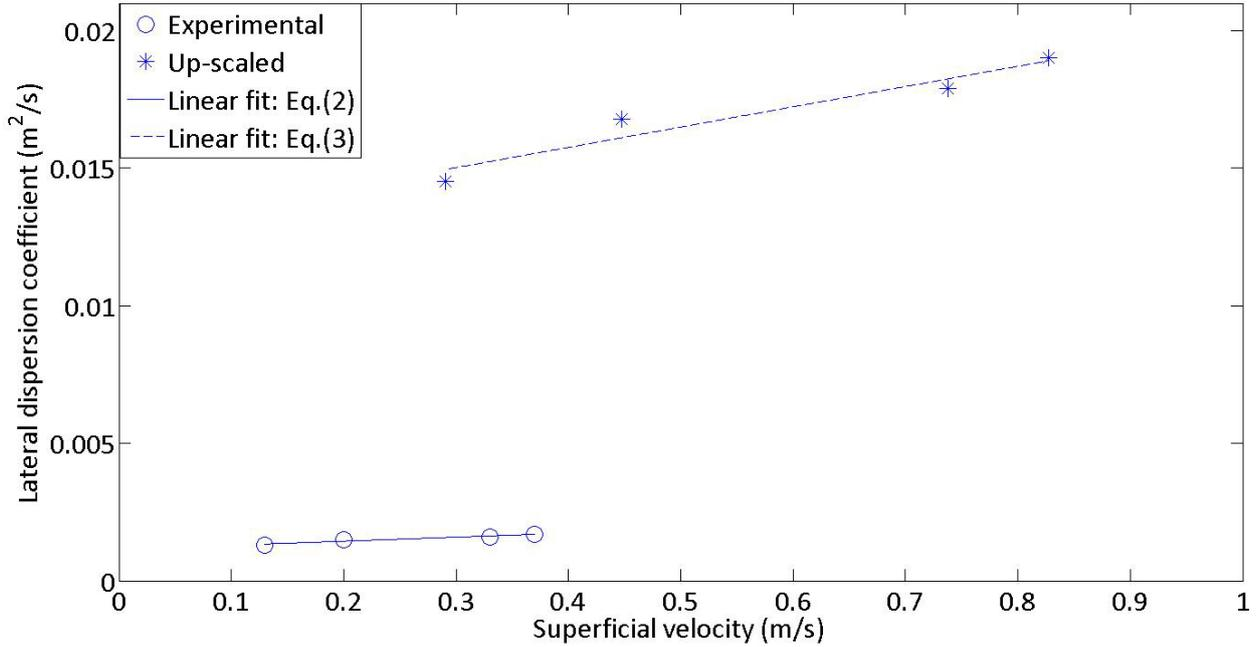
Figure 4: Lateral dispersion coefficients for different velocities from experiments, as measured and recalculated back to large-scale conditions.
