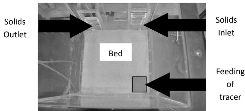
Figure 2: A picture of the cold unit used in the experiments (view from top of unit). The tracer agent is inserted in the bottom-right corner and the concentration was measured over time at the outlet located in the top-left corner.
