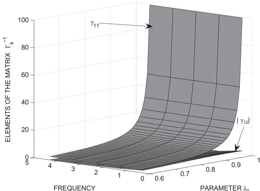
**Fig. 9** Elements of the matrix  $\Gamma_k^{-1}$ . The diagonal entry  $\gamma_{11}$  and non-diagonal entry  $|\gamma_{12}|$  are plotted for  $k = w = 150$  and  $\lambda_1 = 1$  as functions of the frequency  $q$  and forgetting factor  $\lambda_0$ . The diagonal entry  $\gamma_{11}$  is calculated using (43) and non-diagonal entry  $|\gamma_{12}|$  is calculated using (45)
