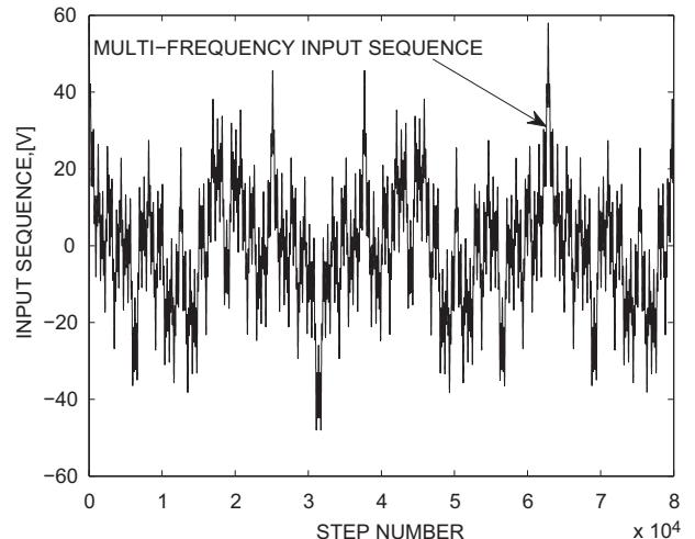
**Fig. 6** The input multi-frequency test sequence  $u_k$  to DC motor is plotted as a function of a step number and specified in a form of trigonometric polynomial  $u_k = \sum_{q=q_1}^{q=q_7} A_q \cos(qk\Delta)$ , where  $A_q = 10, 8, 8, 8, 8, 8$  [V] are the amplitudes at frequencies  $q=3, 7, 15, 25, 45, 100, 300$  [ $\frac{1}{s}$ ] respectively,  $\Delta=0.0001$ ,  $k=0, 1, 2, \dots$
