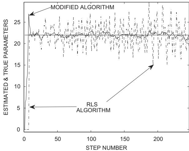
**Fig. 4** System (4), (7) with  $q = 1, 2, 3$ ,  $\sigma^2 = 1$ , was simulated with the modified Kaczmarz algorithm (20), (21) plotted with a solid line and the RLS algorithm (27), (28) plotted with a dash-dotted line. The two estimated parameters converge to the true value which is equal to 22
