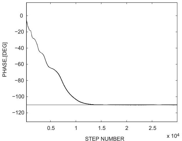
**Fig. 8** The values of the phase  $\psi_{qk} = -\arctan \frac{b_{qk}}{a_{qk}}$  estimated via modified algorithm (20), (21) are evaluated at frequency  $q=3[\frac{1}{\text{s}}]$  and plotted as a function of a step number. A true value of the phase  $\psi_{q^*}$  calculated via (31) is equal to  $-110.13^\circ$
