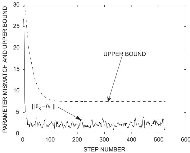
**Fig. 1** Parameter mismatch  $\|\tilde{\theta}_k\|$  and upper bound (22) are plotted as functions of a step number. The system (4), (20), (21) with the parameters  $\lambda_0 = 0.95$ ,  $\lambda_1 = 1$ ,  $\gamma_0 = 10$ ,  $q = 1, 2, 3$ ,  $\sigma^2 = 3$ ,  $c_\xi = 3\sigma$  was simulated
