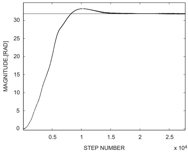
**Fig. 7** The values of the magnitude  $|\hat{H}(iq)| = \frac{B_{qk}}{A_q}$  estimated via the modified algorithm (20), (21) are evaluated at frequency  $q=3[\frac{1}{\text{s}}]$  and plotted as a function of a step number. A true value of the magnitude  $|H(iq)| = \frac{B_{q^*}}{A_q}$  calculated via (30) is equal to 31.87
