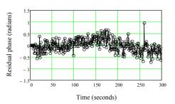
Figure 3: Residual phase of the fringe. Clock offset calibration accuracy is at a level of 0.2 ns, clock rate offset determination accuracy is better than 0.05 ps/s. Phase noise is at a level of 0.2 radians at 1 s sampling.
