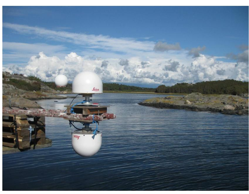
modified to emphasize Left-Handed Circularly Polarized energy from below the horizon. Both the UP and DOWN receivers were tracking at 1-Hz. Rather than a geodetic installation, where the antenna is pounded into bedrock, these antennae have been deliberately set above the local sea surface. There was no *in situ* tide gauge at OSO during the period of this experiment, September-December 2010. However, tide gauges at Ringhals (18 km) and Göteborg (33 km) are available for comparison.
