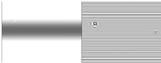
Figure 10. Synthetic radiograph (1024x1024 pixel) of a typical weld and its wavelet filtered version with K=7 using a Daubechies filter of order 14. The left is brightness-contrast optimized for showing both pores at the same time, and the right image is optimized for showing also the none-pore noise.
