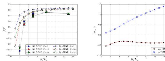
FIGURE 3: Scaling of  $PF_Z$  with **electron density gradient** ( $R/L_{n_e}$ ) shows saturation for peaked profiles, despite increased QL growthrate. A flux reversal is observed with both QL and NL for flat background density profiles.
