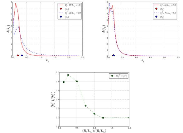
FIGURE 5: The  $k_{\perp}$  spectra of the impurities show a shift toward larger  $k$ , when  $R/L_{n_Z} < R/L_{n_e}$ . The trend is investigated by measuring the quotient between the mean  $k_{\perp}$  of impurity and main ions, as a function of  $(R/L_{n_Z})/(R/L_{n_e})$ .
