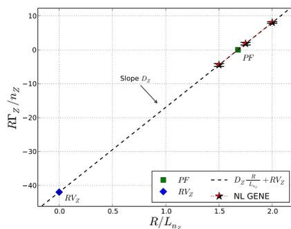
FIGURE 1: The **impurity flux dependence** on  $\nabla n_Z$ , illustrating  $PF_Z$  and the validity of the linearity assumption (3) of equation (1) for  $\Gamma_Z \sim 0$ , and how the parameters of equation (3) are estimated. Data from NL GENE simulations.
