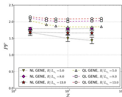
FIGURE 2: Scaling of  $PF$  with **impurity charge** ( $Z$ ) shows saturation for heavy impurities.
