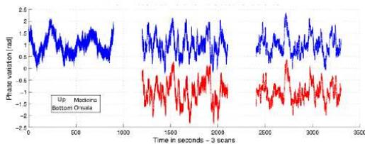
**Fig. 3** Phase fluctuations for the three: GLONASS satellites PR11, PR21, PR13 observed at Medicina (top) and Onsala (bottom).
