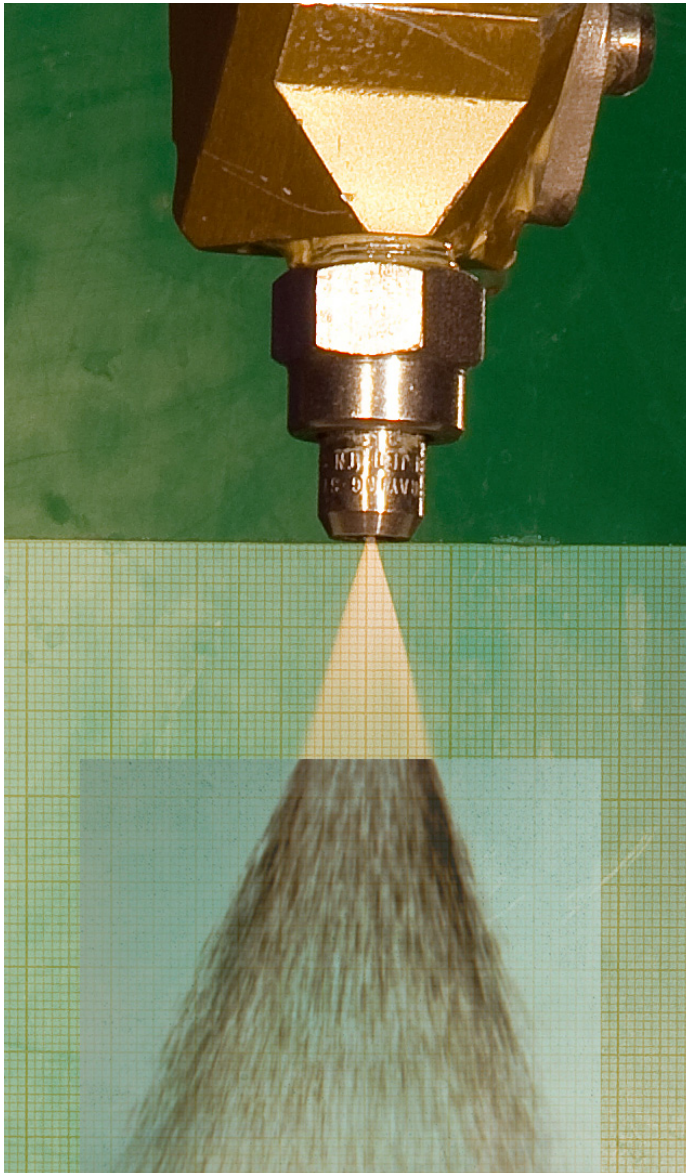
Figure 11: Stationary applicator with sealing droplets visible. Millimeter scale in the background.
