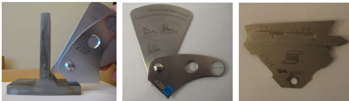
Figure 2: a) Measurement principle audit gauge, a-height [mm], b) audit gauge – calculates a-height from measured position of weld toe, c) production inspection gauge, measure a-height directly on weld ridge (45 deg from base plate).
