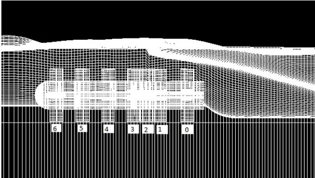
Figure 5: Propeller positions from pos0-pos6; Pos6 is the aft most one
