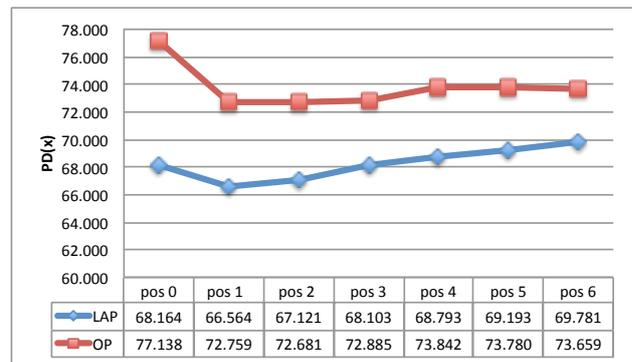
Figure 16: Variation of delivered power with propeller position; LAP vs OP
