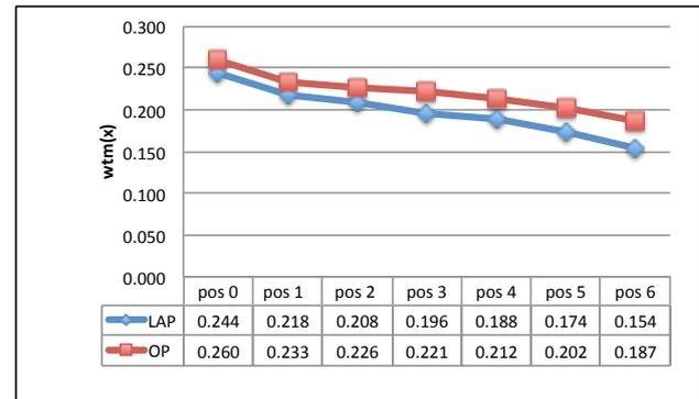
Figure 7: Variation of  $w_{tm}$  with propeller position; LAP vs OP
