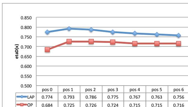
Figure 15: Variation of total propulsive efficiency with propeller position; LAP vs OP
