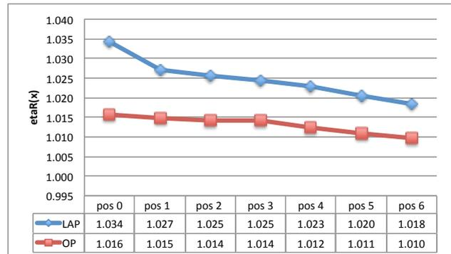
Figure 12: Variation of relative rotative efficiency with propeller position; LAP vs OP
