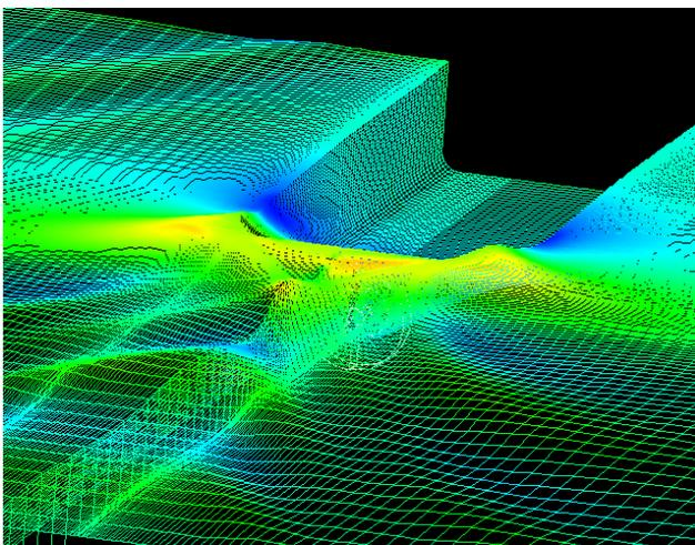
Figure 4: Wavy surface and RANS grid
