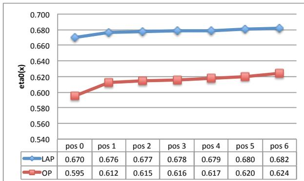
Figure 15: Variation of propeller efficiency with propeller position; LAP vs OP
