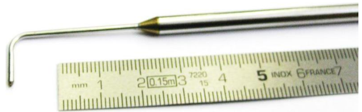
Figure 6: The 5-hole probe used in the measurements
