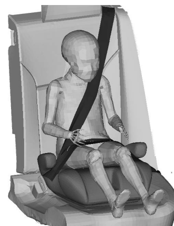
Figure 3. The THUMS 3-year-old model in an optimal sitting posture restrained by seat belt in the rear seat using a backless booster (Andersson et al. 2011a)
