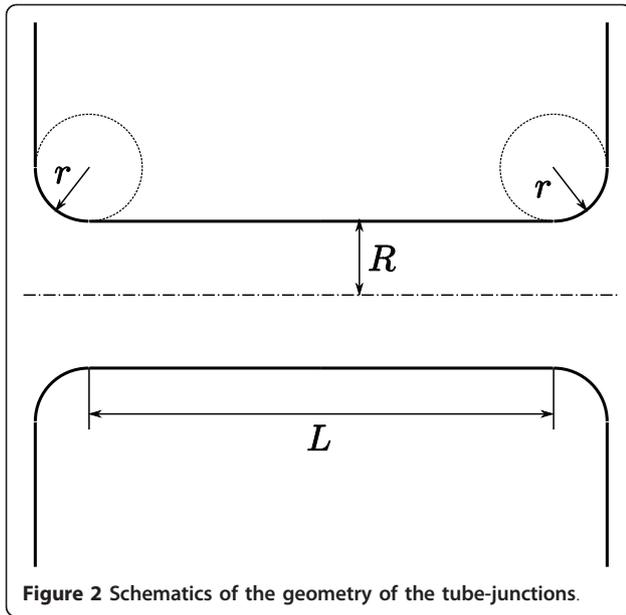
**Figure 2** Schematics of the geometry of the tube-junctions.
