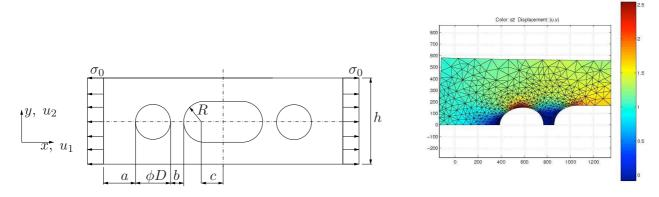
Figure 1: Left: plate with three holes. Right: the color represents the stress distribution in a quarter of the plate. The largest principal stress is presented. The applied stress is  $\sigma_0 = 1$ . Note the higher stress near the holes and the mesh refinement around the holes. Note also the deformed geometry.
