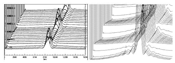
Figure 2. Temporal evolution of spectra for GLONASS satellites PR17 (left) and PR03 (right) observed at Medicina. In a right-hand-coordinate system the X-axis shows frequency, the Y-axis time, and the Z-axis signal strength in arbitrary units. These spectra cannot be compared directly to the ones observed at Onsala shown in Figure 1. Strong variations in signal strength become clearly visible.
