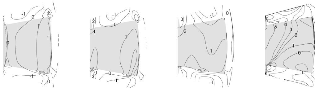
Figure 10: Radial velocity components [ m/s ] just above the rotor pole: Case 1 (left), Case 2 (center left), Case 3 (center right) and Case 4 (right)
