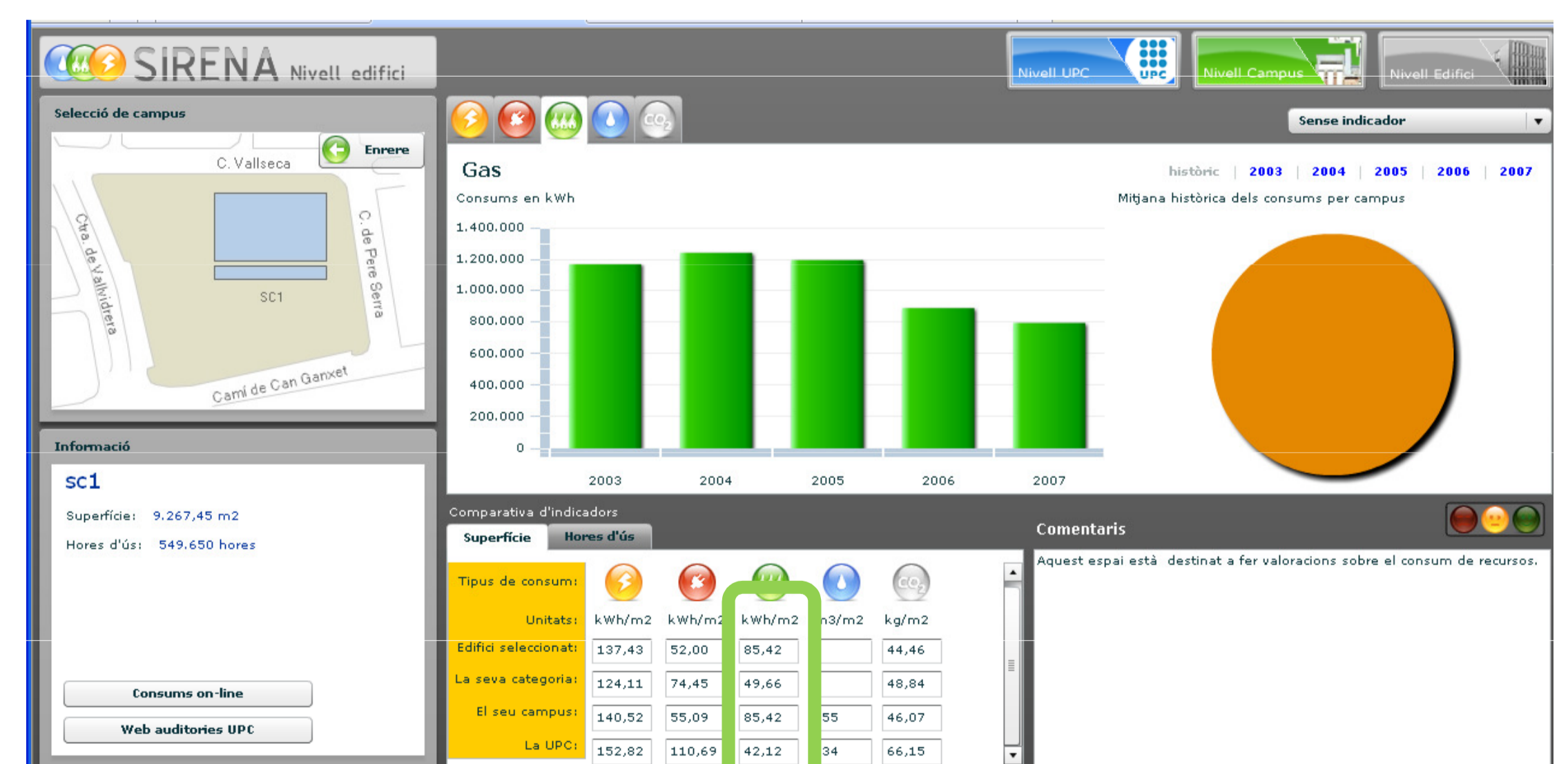
Figure 5. Calculated consumption for heating for O1 (76.6 kWh/m 2 y) fits the range of measured indexes (49.6 to 85.4 kWh/m 2 y). Available at: www.upc.edu/sirena .
