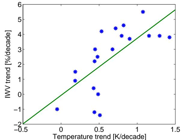
Figure 9. The relation of the estimated IWV trends from the GPS sites in the Swedish GPS network vs. the corresponding estimated trends in the ground temperature at nearby sites. The estimated linear relation (green line) has a slope of 3.8%/K.
