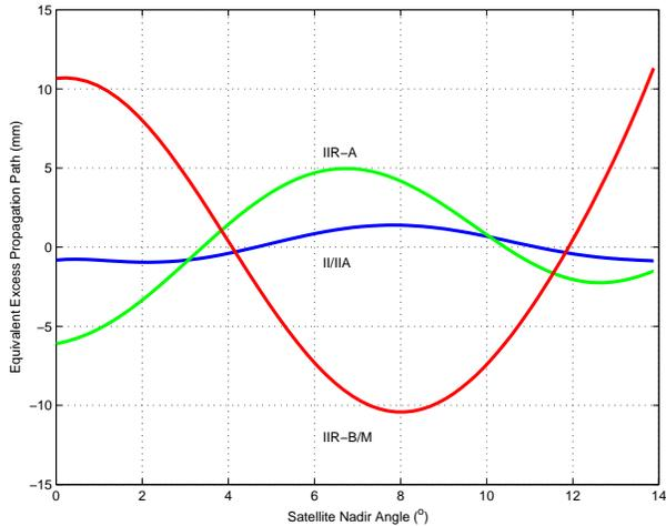
Figure 6. Antenna phase center variations vs. the nadir angle from the satellite to the ground receiver for the three satellite types II/IA (blue), IIR-A (green), and IIRB/M (red) (from [9]).
