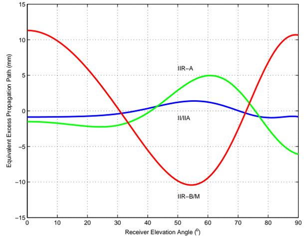
Figure 7. Antenna phase center variations vs. the elevation angle of the satellite seen from the ground receiver for the three satellite types II/IA (blue), IIR-A (green), and IIRB/M (red) (from [9]).
