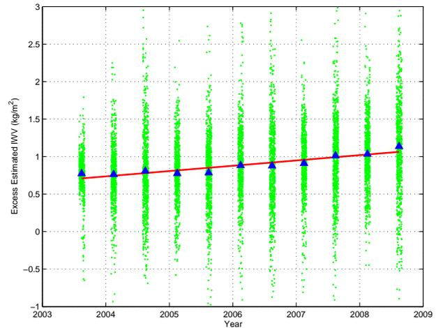
Figure 8. Difference in estimated IWV between two GPS solutions: with and without the antenna (both the satellites and the receiver) phase centre corrections applied. The blue triangles illustrate the mean values for each month. The red line in the figure is the least squares fit to the estimated IWV differences and has a slope of  $0.7 \text{ kg/m}^2/\text{decade}$  (from [9]).
