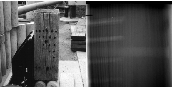
Figure 4: Simulated deterioration that caused loss of cross section results in an deviation of the greyscale on the X-ray image [1].
