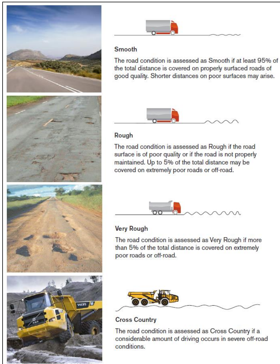
Figure 5-5: Four typical road types, whereof the upper 3 can be considered as road types. From (AB Volvo, 2011).
