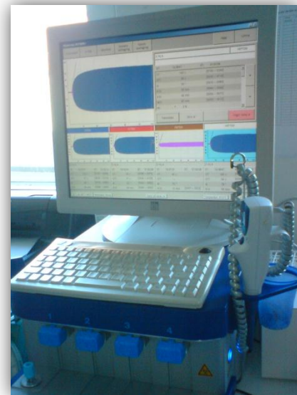
Figure 2.5 The ROTEM ® device. Below, the four channels for blood analysis can be seen as blue blocks. To the right, there is an electronic pipette, and on the screen the results from the analysis can be viewed.
