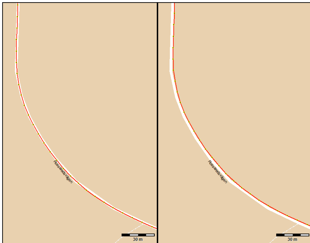
Figure 4.7 Two spline interpolations. The left picture without the right-hand traffic modelling algorithm and the right picture with the algorithm turned on.
