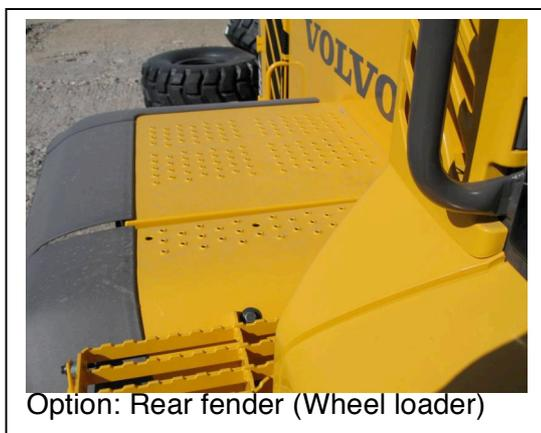
Figure 18. Detailed picture of the possible location of ESS on the wheel loader.
