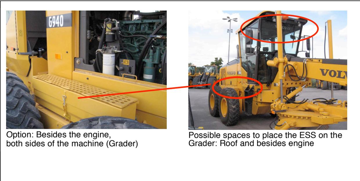
Figure 19. Detailed pictures of the possible locations of the ESS on the grader.
