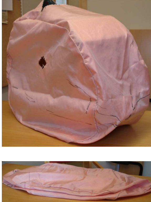
Figure 5: “Inflated” and flat folded passenger airbag.
