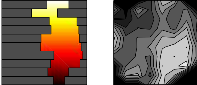
Figure 6: Snapshot of the motion of the multileaf collimators (left figure) for the fluence (intensity) profile shown in the right figure for a cross-section of the beam.
