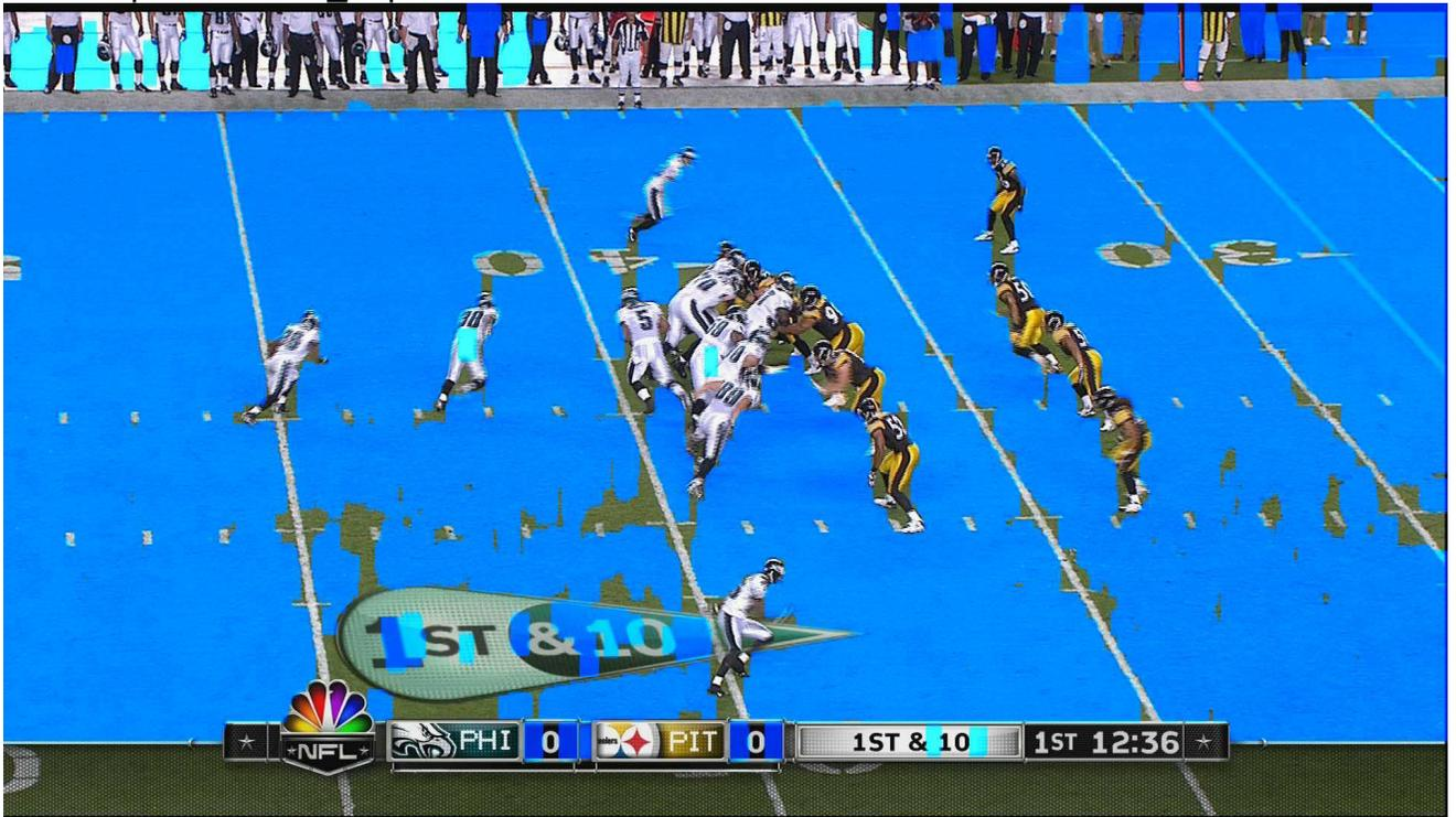
*Figure 5.1 The first 65% lowest activity pixels are dyed in blue (overlapped block size: 16x16)*
