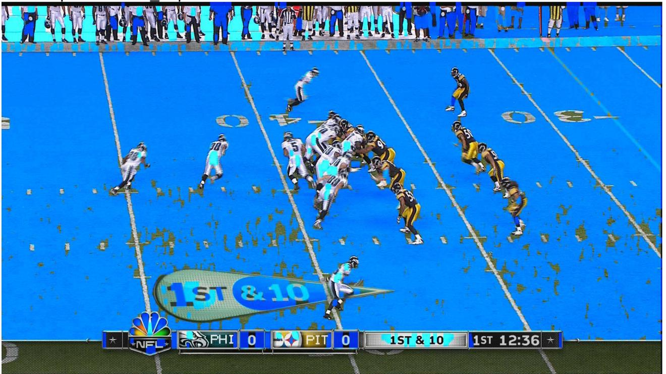
*Figure 5.2 The first 65% lowest activity pixels are dyed in blue (overlapped block size: 8x8)*
